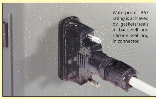
Mate connectors and secure backshell thumbscrews to threaded jackscrews.
